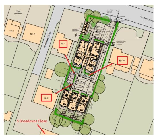
Proposed site plan showing relationship with neighbouring properties (45 degree lines marked in red)
